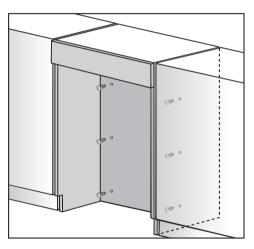
screw the back wall of the cabinet in several places directly to the wall behind it.
